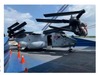
Commercial. *Endurance* is one of the largest Roll-on Roll-off (Ro-Ro) ships in the world with an overall length of 868 feet (264 meters) and is one of only a handful of U.S.-flag Ro-Ro ships capable of and certified to carry V-22s. The vessel has a stern ramp capable of carrying loads weighing up to 320 metric tons (MT), a main deck maximum height of 20.50 feet (6.25 meters), and 262,000 square feet of militarily useful capacity.
