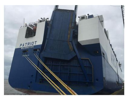
M/V Patriot is 199m long with a beam of 32.26m. She has a 14.15m wide and 7.04m high stern opening, with a stern ramp rated for cargo up to 240 MT.
